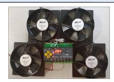
Fan Failure and Temperature Detection Unit (FFTDU) CMSC – 7933 is an integrated intelligent programmable & compact unit, designed to ensure monitoring of 4 Nos. of <u>AC impedance protected cooling fans &Capacitor driven FANS & internal panel temperature in a most cost effective and reliable way for FAN currents from 100ma to 450ma.</u>
