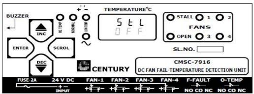
3. If you press ENTER, previously programmed Auto Relay OFF enable/disable status will be displayed on the front panel as shown below
