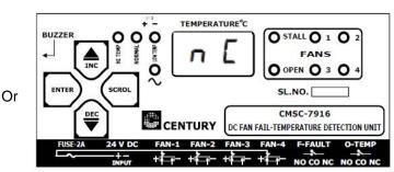
5. Use INC or DEC key to change between NO and NC relay operation types and press ENTER to store.
