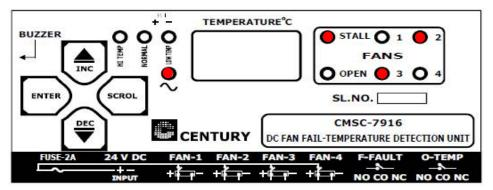
As an option, if a particular fan gets stalled, then the particular relay powering that fan can be put OFF to save energy which would have otherwise been heating the stalled fan. However, there is an option to recheck the particular stalled FAN at programmable time interval (6 sec to 120 sec). At the expiration of each programmed interval, the respective FAN Relay will be put ON to check if the fan is still stalled or running normally. See section 2.1.4 to know how to program this feature.
