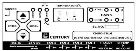
6. Now previously programmed Stall Recheck time will be displayed on the front panel with its first digit blinking as shown below.
