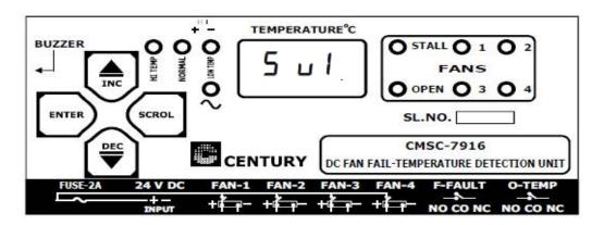
2. Press SCROL key 9 times to scroll through Fn1 – F4 enable / disable status and Fan type (or continue from #10 of sec 2.1.3) and go to Auto RELAY OFF option. You will see 'S t L' and 'O F F' toggling on the front panel as shown below.
