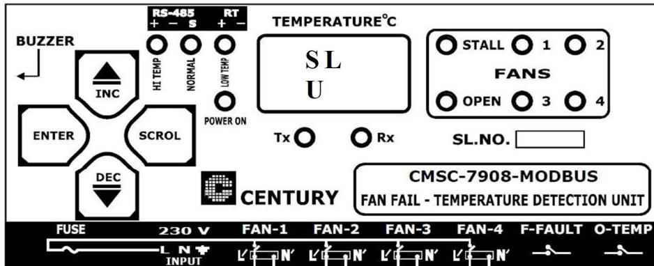
2. Press SCROL key 9 times to scroll through Fn1 – F4 enable / disable status ( or continue from #7 of sec 2.1.3) and go to 'Fans type' parameter. You will see 't Y P' on the front panel as shown below.
