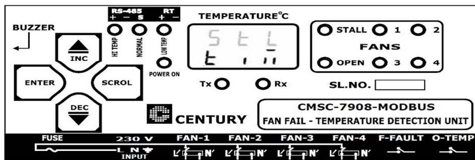
6. Now previously programmed Stall Recheck time will be displayed on the front panel with its first digit blinking as shown below.
