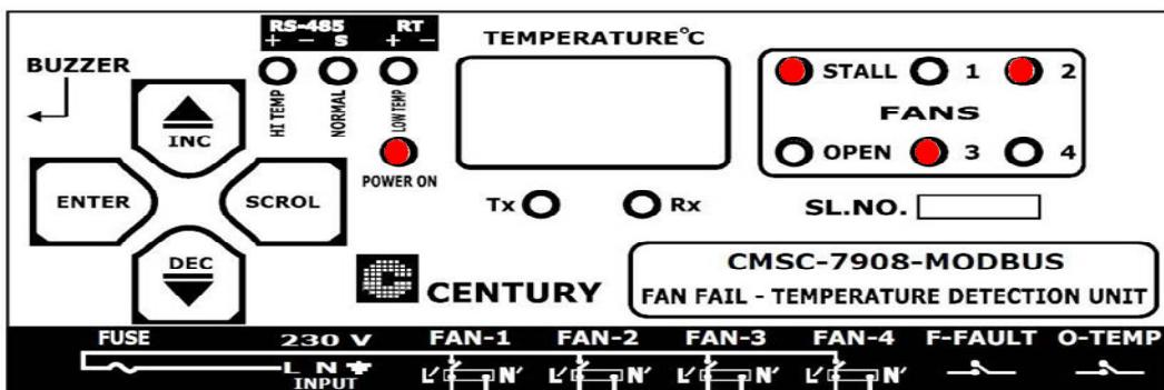
As an option, if a particular fan gets stalled, then the particular relay powering that fan can be put OFF to save energy which would have otherwise been heating the stalled fan. However, there is an option to recheck the particular stalled FAN at programmable time interval (6 sec to 120 sec). At the expiration of each programmed interval, the respective FAN Relay will be put ON to check if the fan is still stalled or running normally. See section 2.1.4 to know how to program this feature.
