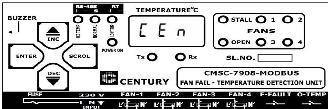
Then the ambient temperature will be displayed on the front panel as shown below.
