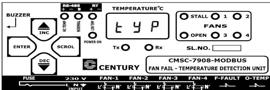
9. If you press ENTER, previously programmed Fan type will be blinking on the front panel as shown below
