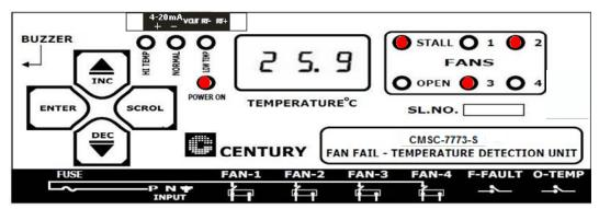
As an option, if a particular fan gets stalled, then the particular relay powering that fan can be put OFF to save energy which would have otherwise been heating the stalled fan. However, there is an option to recheck the particular stalled FAN at programmable time interval (6 sec to 120 sec). At the expiration of each programmed interval, the respective FAN Relay will be put ON to check if the fan is still stalled or running normally. See section 2.1.4 to know how to program this feature.
