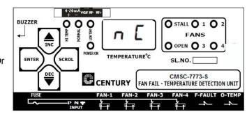
5. Use INC or DEC key to change between NO and NC relay operation types and press ENTER to store.
