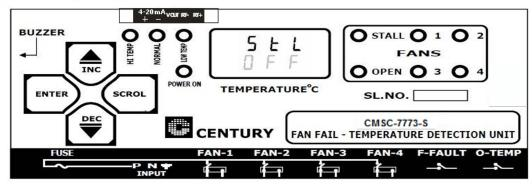
3. If you press ENTER, previously programmed Auto Relay OFF enable/disable status will be displayed on the front panel as shown below
