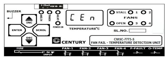
Then the ambient temperature will be displayed on the front panel as shown below.
